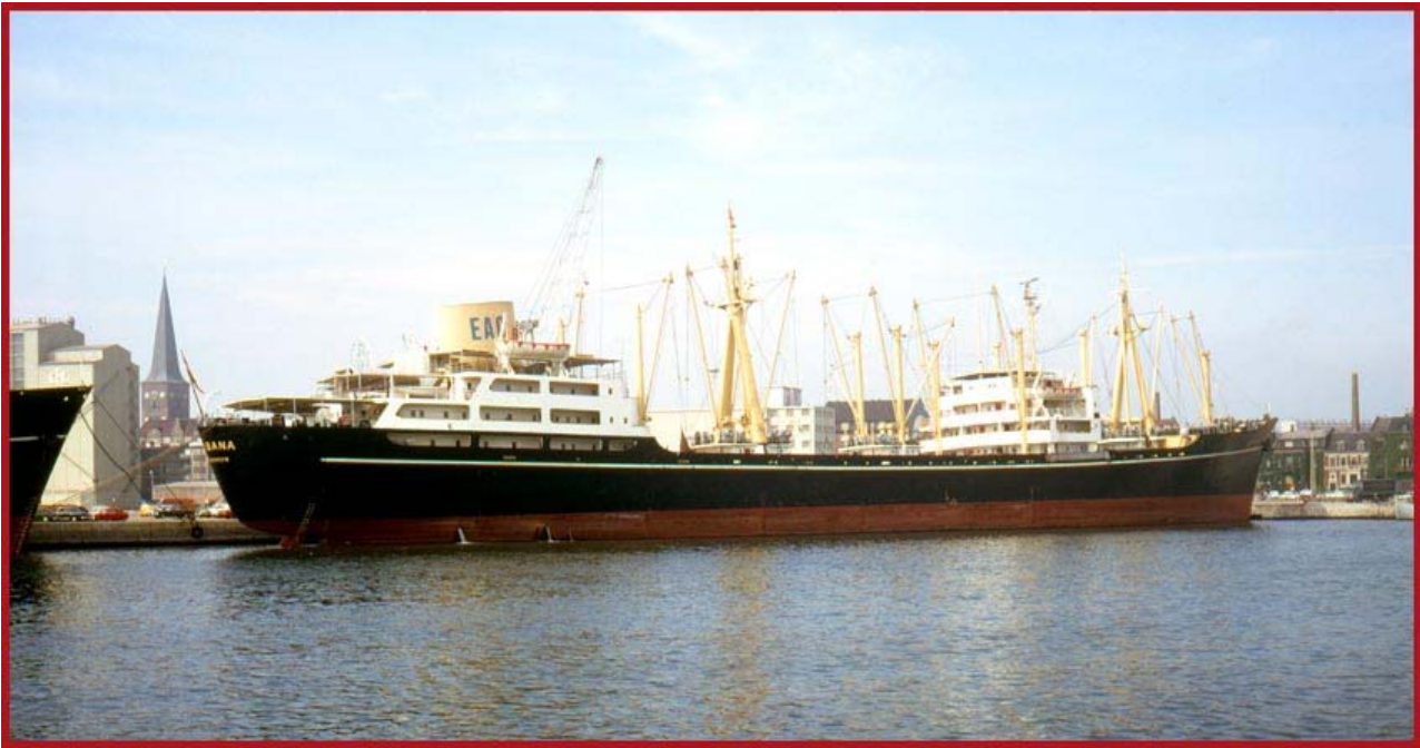
M/S "Boribana" - on this picture, the unusual split superstructure is clearly seen - (Photography by Karsten Petersen)
